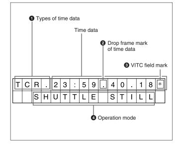
When basic menu item 005 of the setup menu DISPLAY INFORMATION SELECT is set as anything other than OFF, the video signal output from the COMPOSITE (SUPER) output connector, SDI (SUPER) output connector (for J-10SDI/30SDI only) or DV connector contains superimposed character information (overlaid display), including time code, menu settings, or alarm messages.
